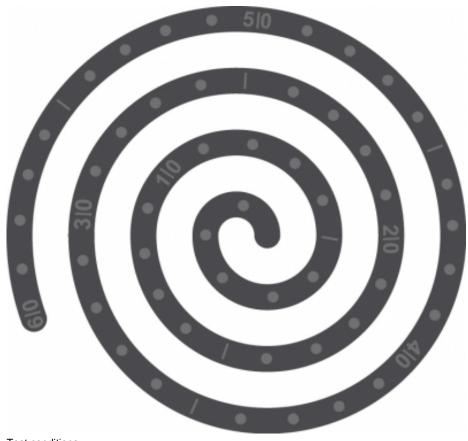
Test conditions: 760 bar (specific pressure) / 200 °C Flow Spiral Dimensions 2 mm x 5 mm
